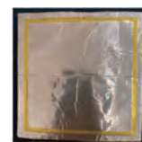
Figure 4. Top view of proximity capacitance sensor
